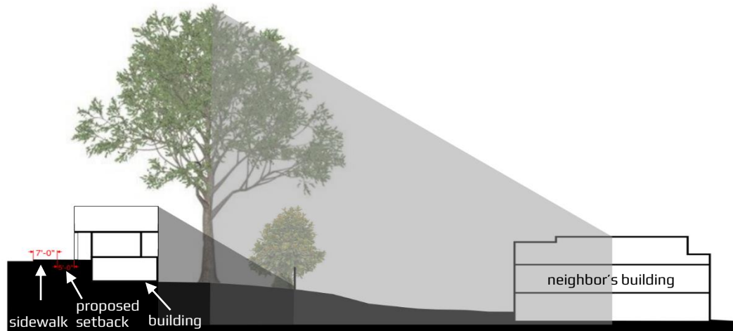
Shadow projection of building with proposed 5ft setbacks @ A-A' section
