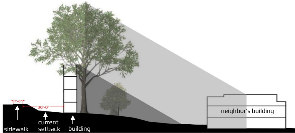
Shadow projection of building with current 30 ft setbacks @ A-A' section
