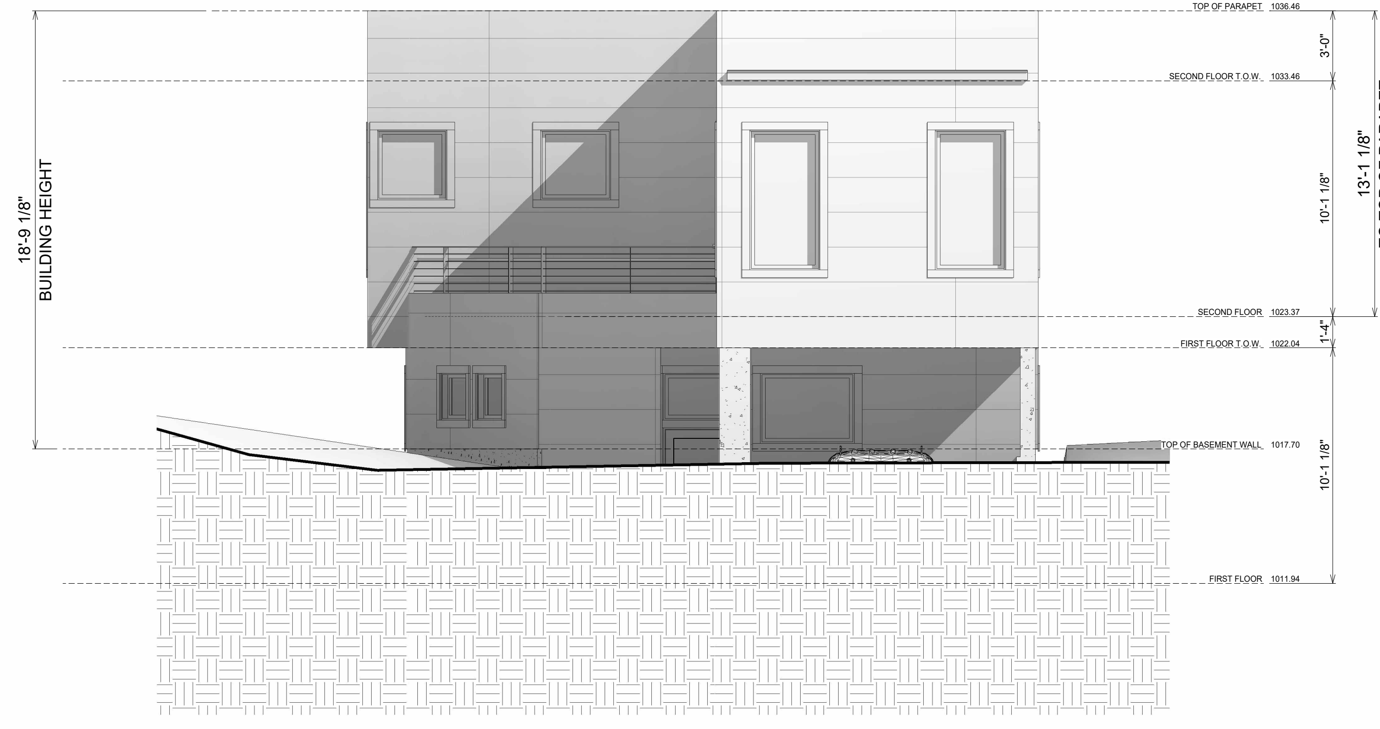
① FRONT ELEVATION 1/4" = 1'-0"
