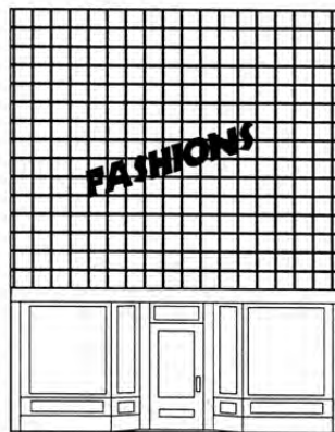
Covering a building’s materials and ornaments robs it of its historic character as seen here. This is inappropriate.
